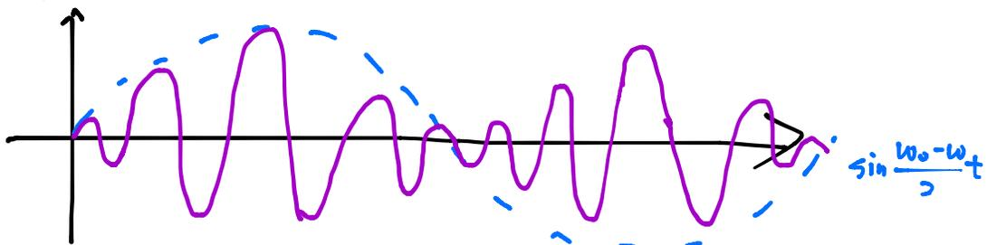
Such vibration is referred as "beats". Can be used to tune the acoustics.
